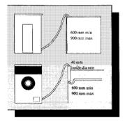
Important: Before connecting up the machine to new pipework or to pipework that has not been used for some time, run off a reasonable amount of water to flush out any debris that may have collected in the pipes.
